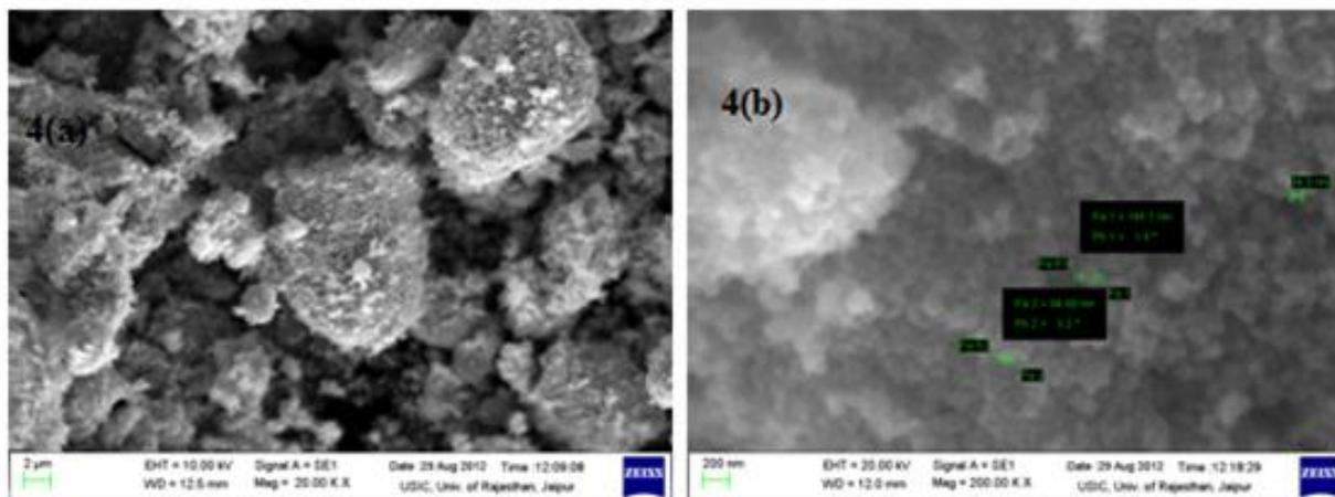
Fig. 4(a) and 4 (b) SEM images of THF mediated ZnO nanoparticles
