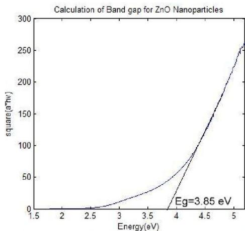
Fig. 2 Bandgap estimation of THF mediated ZnO nanoparticles
