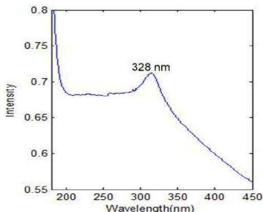
Fig. 1 UV- Vis absorption spectroscopy curve of the ZnO(THF) particles
