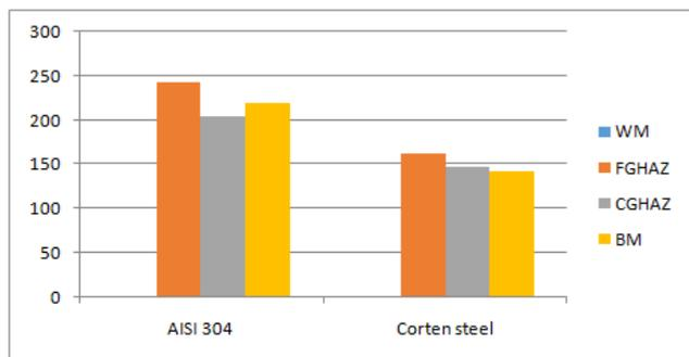
Fig. 5.7. Chart represents hardness at different region of welded sample
