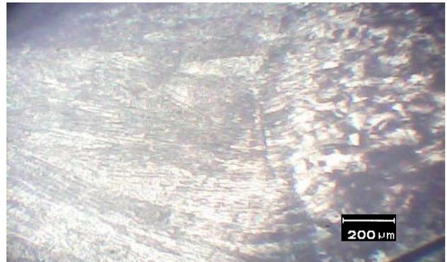
Fig. 5.4 Weld interface to corten steel (100X)
