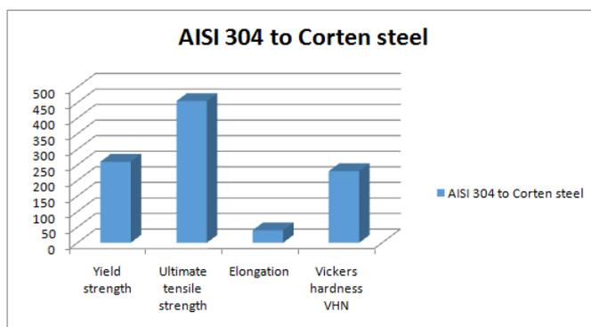
Fig. 5.9. Chart for Transverse tensile properties of the weld joint
