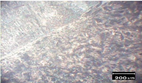
Fig.5.3 Weld interface to SS 304 (100X)
