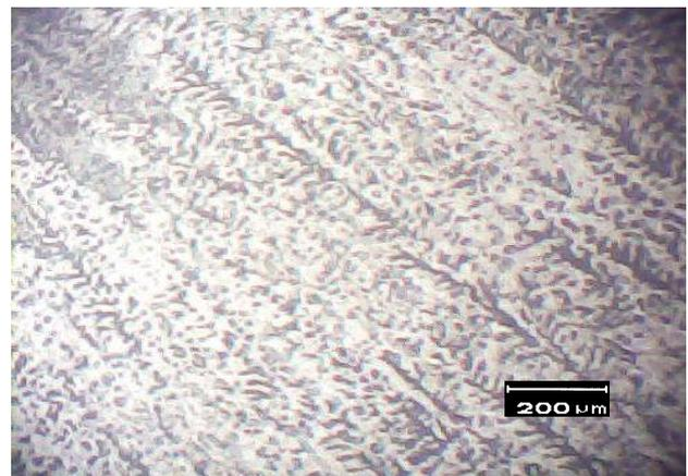
Fig. 5.5. Microstructure of weldment (100X)
