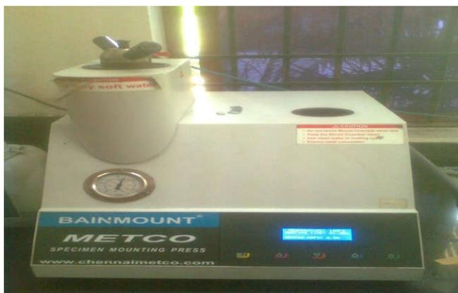
Fig.4.7. Sample mounting machine
