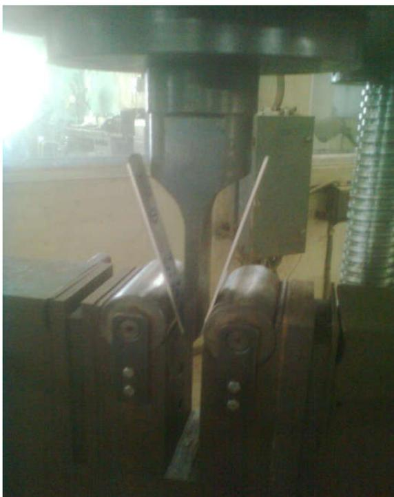
**Fig. 5.11. Bending at final stage**
