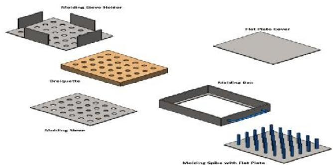
Fig. 1. The component unit of biomass briquette mould
